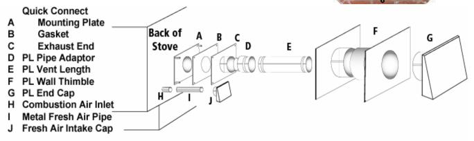
NOTE: Some horizontal, through the wall installations may require a Clean-Out Tee and a minimum 3' vertical rise of pipe inside or outside the building to help draft the stove. This is required if a proper burn cannot be maintained, after the stove has been tested and the airflow set. This is due to backpressure in the exhaust, caused by the airflow around the house.
